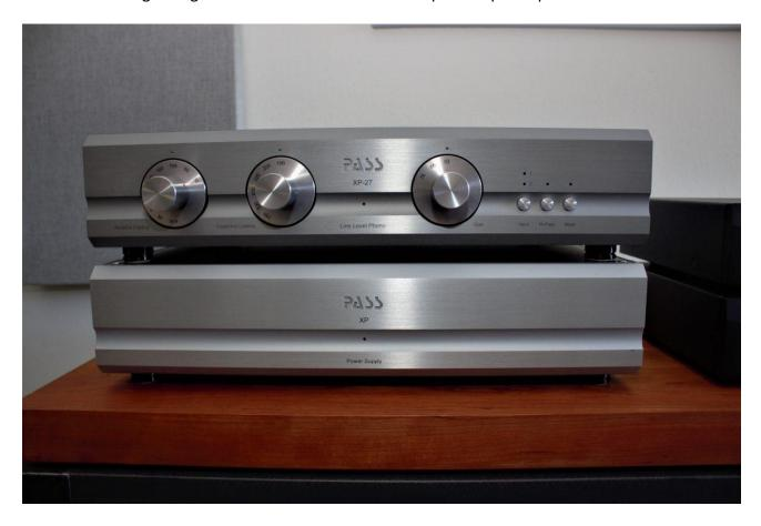
The XP-27 phono preamplifier, like the XP-22, was designed primarily to reduce distortion and noise in the signal path. "Switching and loading is done at higher signal levels," the Pass website proclaims, which improves dynamics, minimizes noise and improves low-level performance. (Both the XP-22 and XP-27 excelled at providing plenty of music information at relatively low volumes.)
